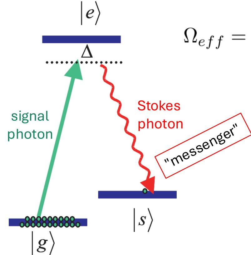
Fig. 11: (coherent) Raman transition
