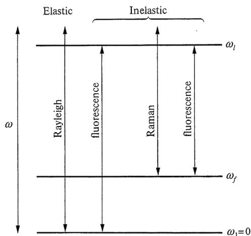
Figure 7: Types of scattering: elastic Rayleigh, inelastic fluorescent, Raman and fluorescent Raman. Incident frequency here is  $\omega$  on the very left [19].
