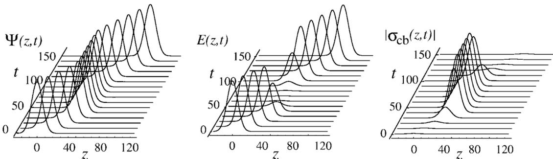
Figure 6: The superposition  $\hat{\psi}$  (left), its photonic part (middle) and its spin-wave part (right) [18]. From the slope of the graph we can see the slow speed of the photonic part and the stationary spin-wave part of the superposition.
