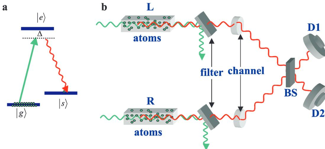
Figure 9: Creating entanglement between two memories. (a) the Raman transition – signal green and Stokes squiggly red, (b) a scheme of the experiment [22].
