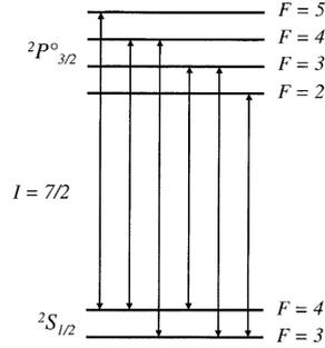
Figure 2: Hyperfine structure with allowed transitions of the  $^{133}\text{Cs}$  ( $I = 7/2$ )  $D_2$  line [11].
