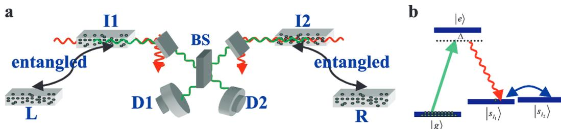
Figure 10: Entanglement swapping between two entangled memory pairs. (a) the scheme of the experiment –  $R$  from one previous pair is  $I_1$ ,  $L$  from another previous pair is  $I_2$ , (b) the Raman transition – anti-Stokes green and control squiggly red, this one visibly pumped in on (a);  $|s_{I_1}\rangle$  and  $|s_{I_2}\rangle$  represent previous entanglement [22].
