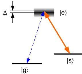
Figure 3: The  $\Lambda$  EIT scheme with detuning  $\Delta$ . Signal is blue and control is orange. [13]
